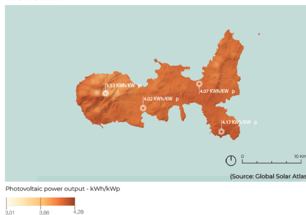
Figure 54: the wind and solar energy potential maps for the Elba island (source Global Wind and Solar Atlas).
